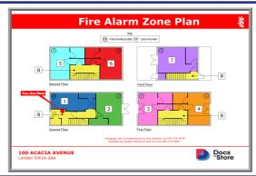
A suitable zone plan of the premises must be provided on or adjacent to all CIE and repeat indicating equipment.
